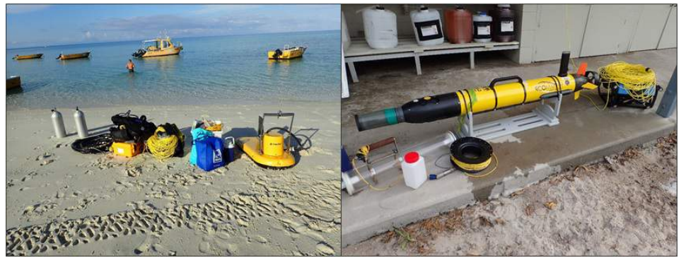
Above: A sea of yellow: Preparing the survey equipment for fieldwork at Lizard Island Research Station; Edgetech sub-bottom profiler. Right: Iver Ecomapper and BlueROV2. © Mardi McNeil
